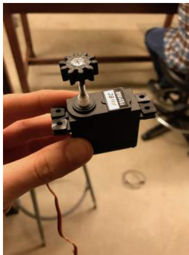
Figure 70: FS106R servo motor with epoxied pinion
