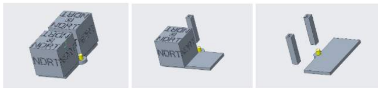
Figure 75: The three phases of the beacon deployment system.
