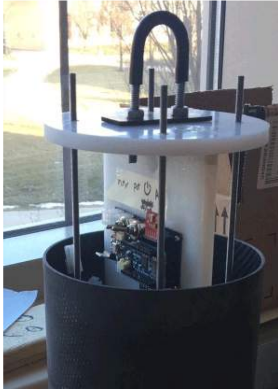
Figure 14: ABS Mount drying inside body tube.
