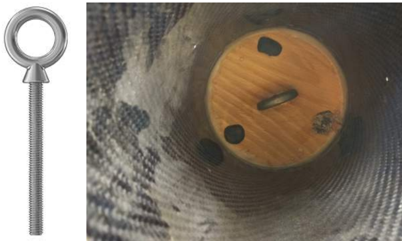
Figure 32: Eyebolt as epoxied into structural bulkheads of launch vehicle
