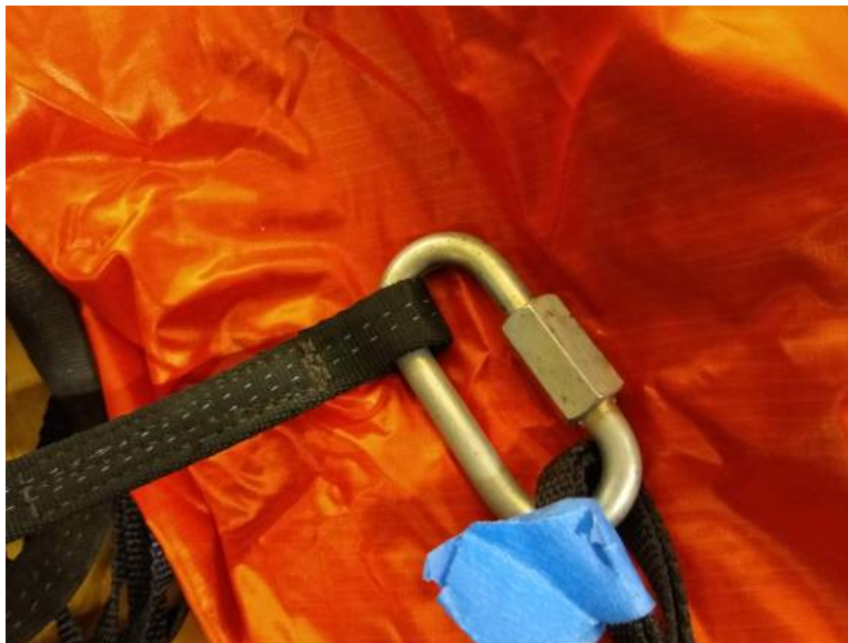
Figure 31: 316 stainless steel quick links used to attach launch vehicle sections to the shock cord
