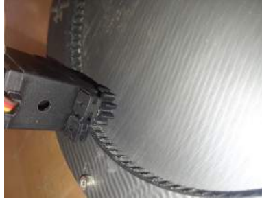
Figure 91: Servo interfacing with ring gear
