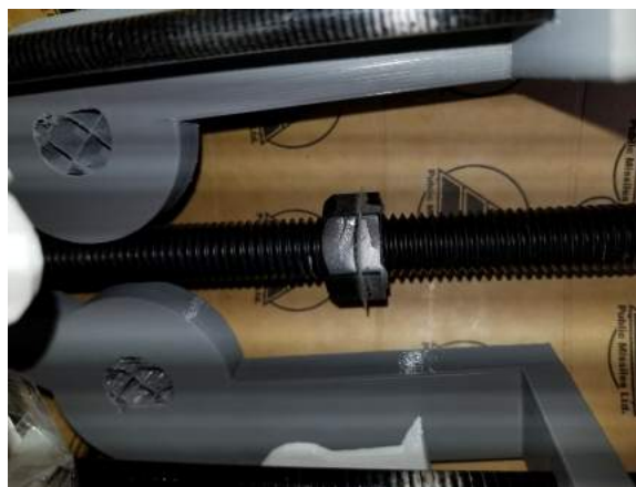
Figure 66: Platform inside the payload bay with broken 3D printed flanges.
