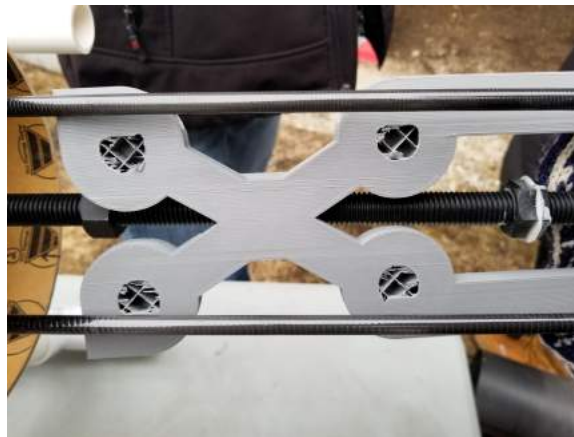
Figure 65: Platform with broken 3D printed flanges.
